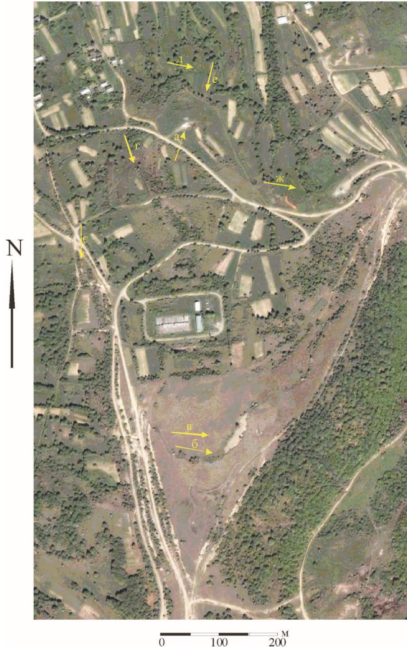
Figure 1 Space photo of the surface in the area of borehole No 10. a - the location of the borehole; б, в - the detachment plane of the "old landslide"; г – deformation terraces on the surface of the landslide relief; д, е - swampy area on the slope from borehole No 10; е - the bedrocks outcrops; ж - sampling for determination of physical and mechanical properties.
